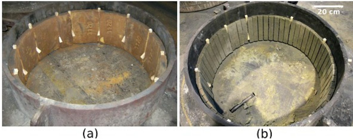
Fig 2: Arrangement of the refractory linings in the ingot feeder heads: (a) traditional RCF linings; (b) innovative linings.
