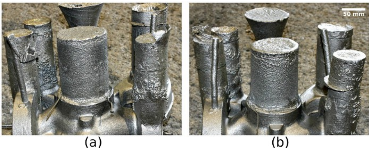
Fig 14: Pictures of investigated foundry castings: (a) endowed with RCF-containing linings and (b) endowed with RCF-free linings.
